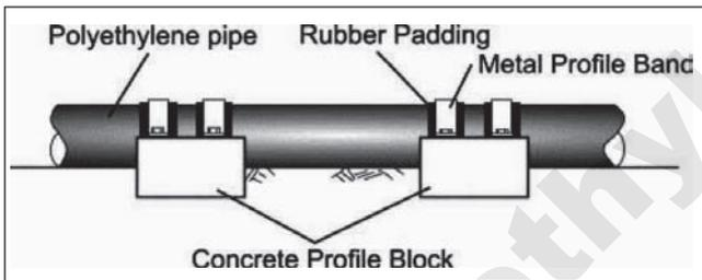
Figure 7 Concrete Cradle or Thrust Block Stabilization
